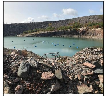
Barrels located in the Broken Hammer open pit are linked to the lime injection system, which is part of the process of treating effluent water before discharge.
